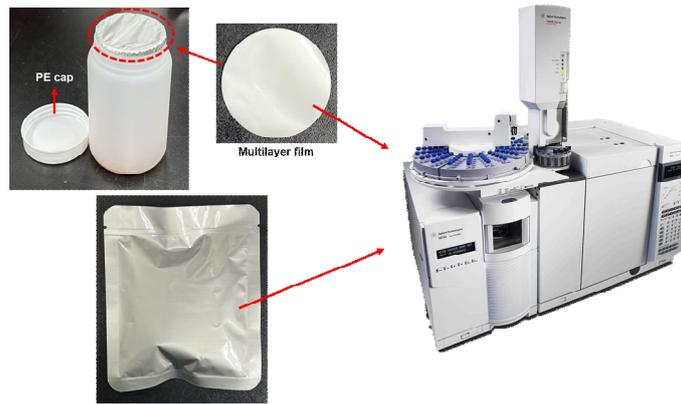
**Fig 3.** The analysis of volatile sulfur-containing compounds of kimchi absorbed in the lid or pouch.
