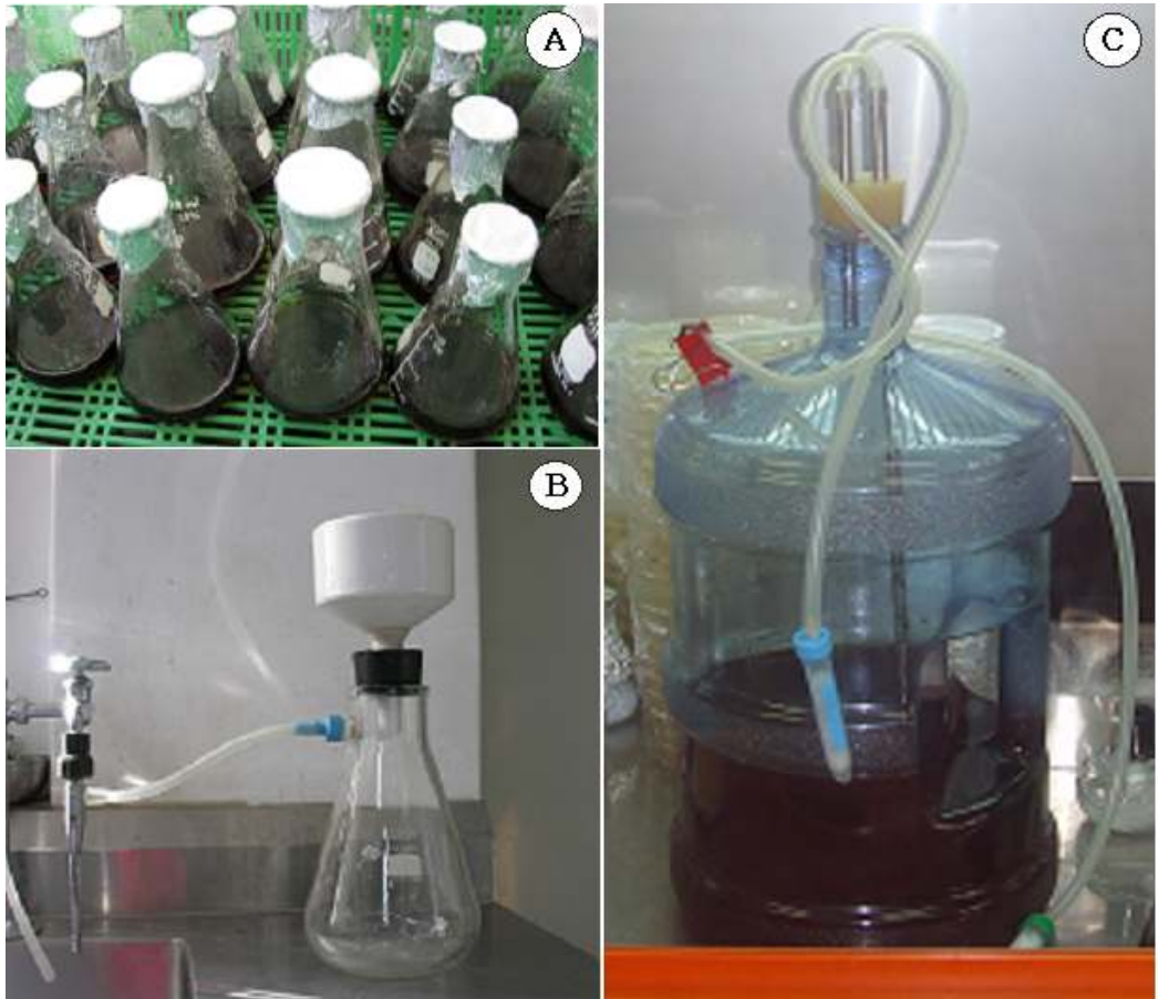
Fig. 1. Fermentation. A. Flask culture, B. filtering system, C. 20 liter fermenter
