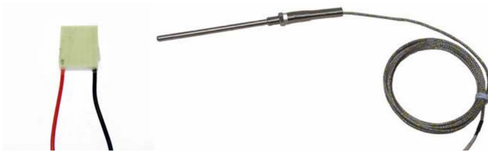
Fig. 6-5 Thermoelectric(left) and Pt-100 RTD(right).
