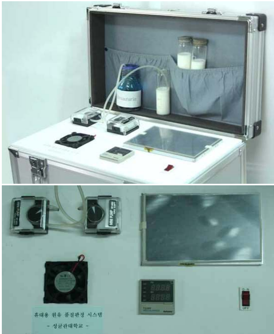
Fig. 6-1 Real time portable quality evaluation system of cow's milk.
