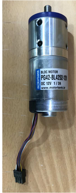
[국산화 Electric Mast 적용 BLDC Motor]
