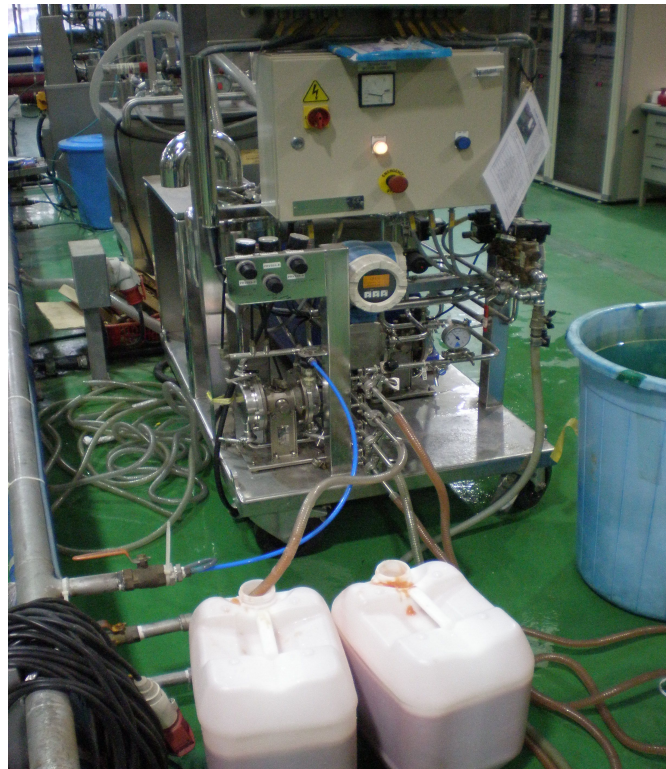
Fig. 13. Two-phase continuous separation of pulp and juice from watermelon
