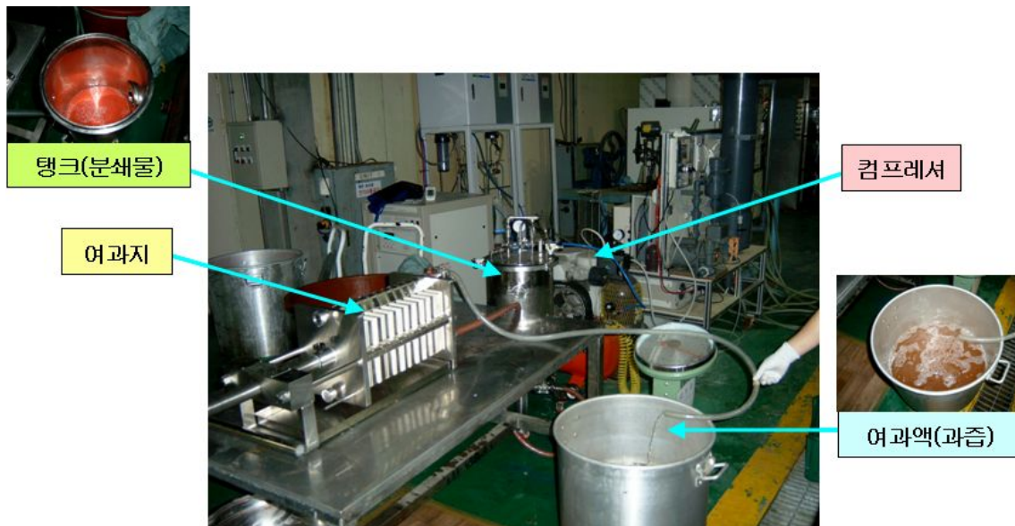
Fig. 12. Separation of pulp and juice from watermelon by using filter press.
