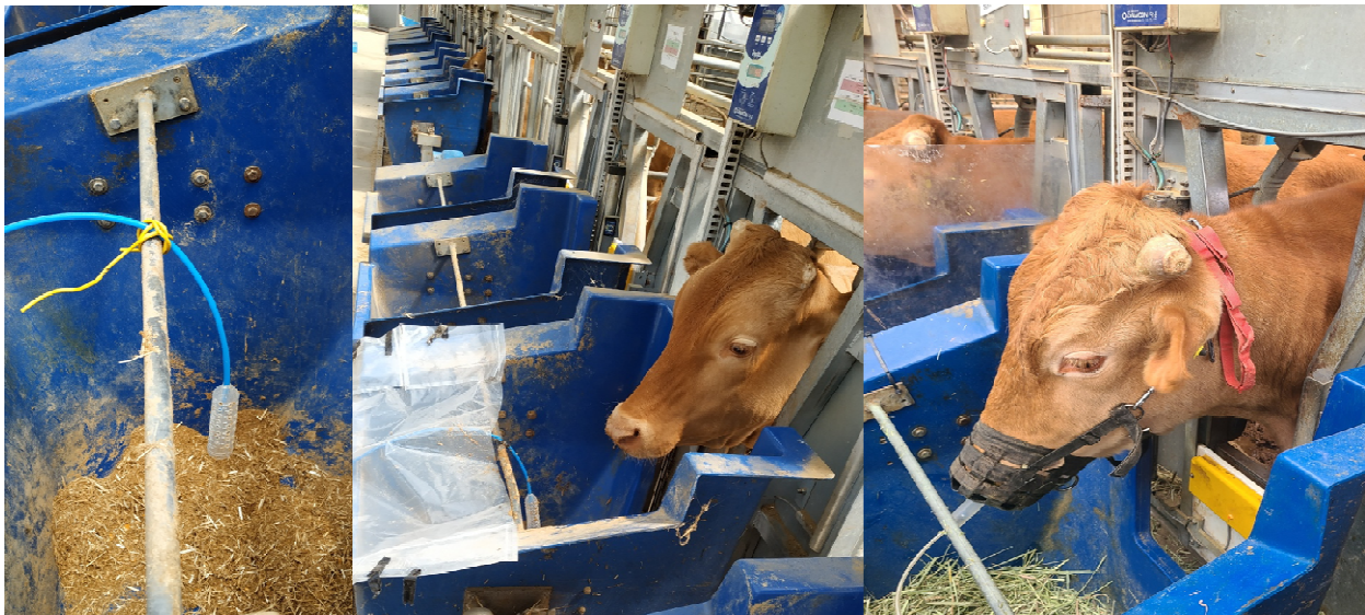
Figure 1-1. The installation of the CO 2 method to compare with respiratory chamber method
