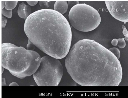
Fig. 95. SEM micrographs of microparticulated (A) Phellinus Linteus , (B) potato starch after sieving, (C) composite, potato starch : Phellinus Linteus = 9:1, (D) composite, potato starch : Phellinus Linteus = 19:1, (E) composite, potato : Phellinus Linteus = 29:1.
