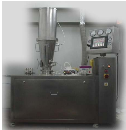
Fig. 6. Fluid Bed processor type FBC -1 Bottom spray system Batch capacity : 1 kg /batch Filter type : polyester , T165P Nozzle insert: 1.2 mm dia Bottom plate : type B.
