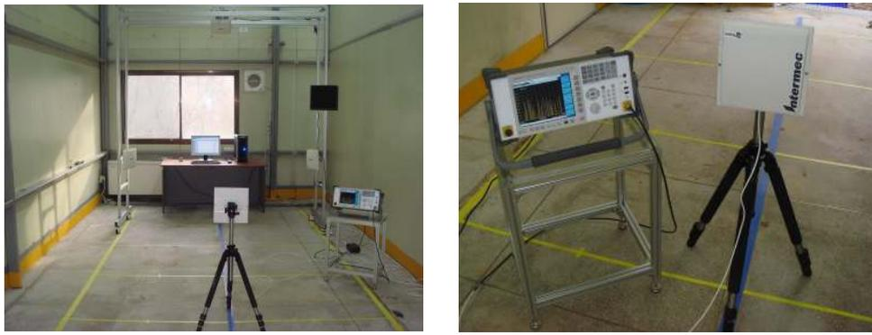
Fig. 3-7 View of test for reader power of gate type RFID system
