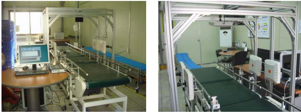
Fig. 3-11 Conveyer type RFID system
