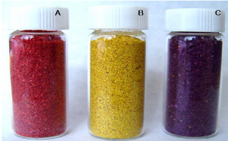
Fig. 1. Powder of freeze dried edible flowers used in experiments.(A : Begonia semperflorens "Superolympia Red", B : Tagetes erecta "Boyorange", C : Viola wittrockiana "Matrix clear purple")
