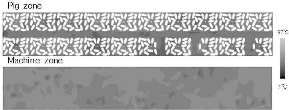
Fig. 80 Temperature distribution according to the height in case 1, pig house B
