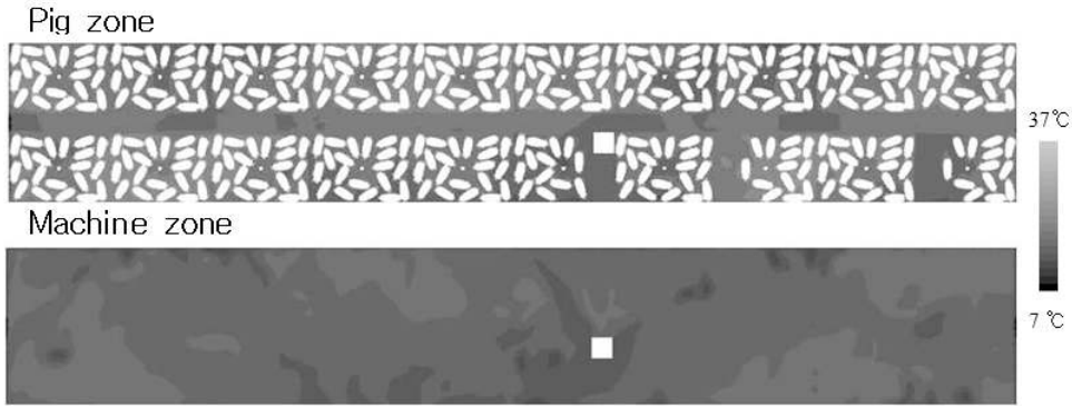
Fig. 95 Temperature distribution according to the height in case 4, pig house B
