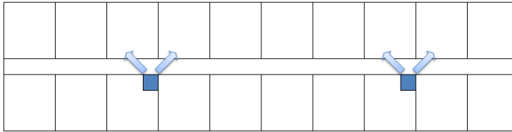
Fig. 128 Location and direction of wet air cleaner in case 5, pig house C
