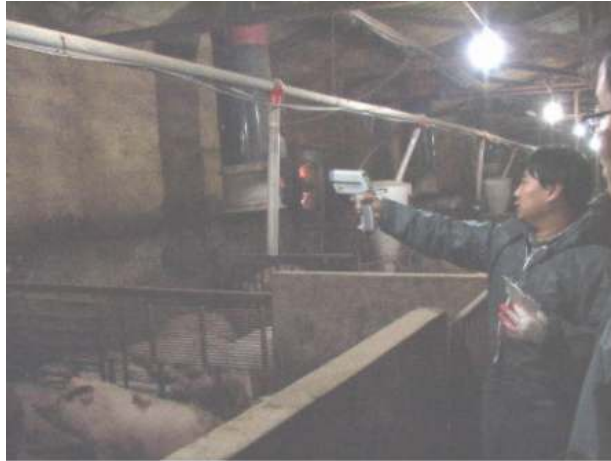
Fig. 19 Measurement of a surface temperature using RAYNGER
