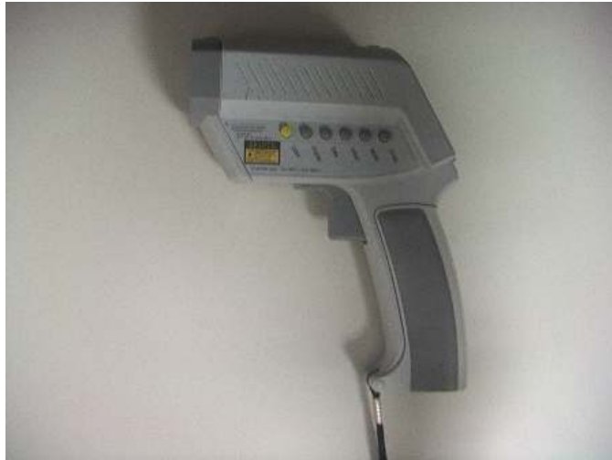
Fig. 4 Infrared gun to measure a temperature of a surface
