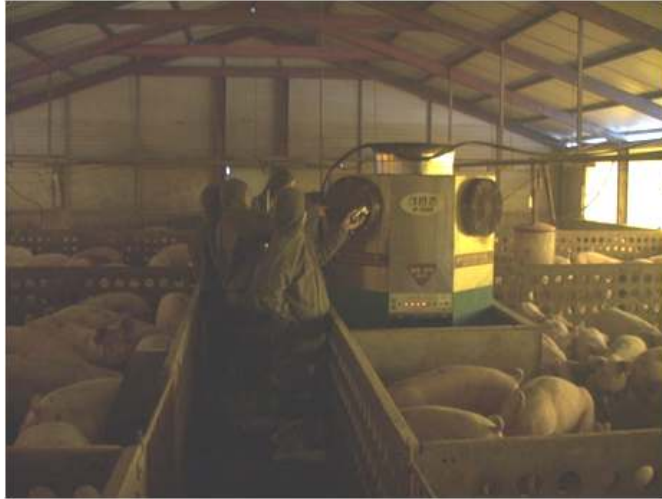
Fig. 21 Experiment of efficiency of wet air cleaner at pig house B
