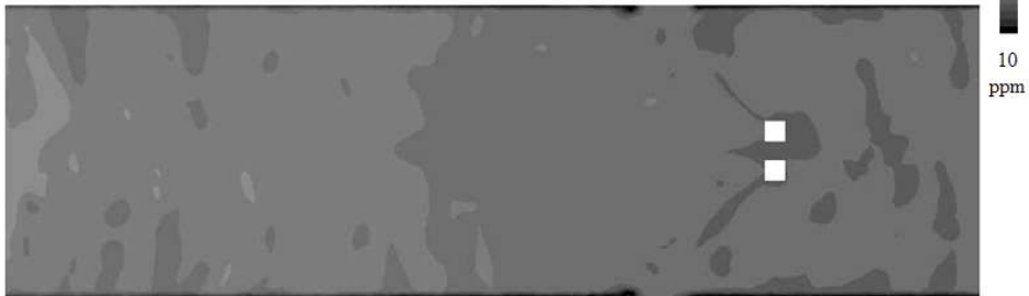
Fig. 136 Ammonia distribution according to the height in case 6, pig house C
