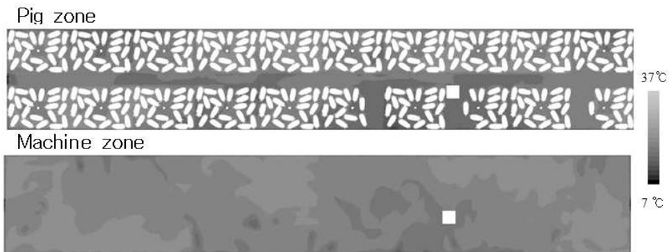
Fig. 105 Temperature distribution according to the height in case 6, pig house B
