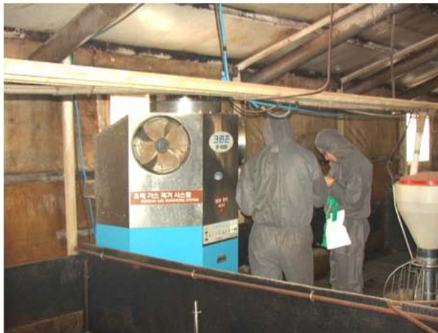
Fig. 20 Experiment of efficiency of wet air cleaner at pig house A
