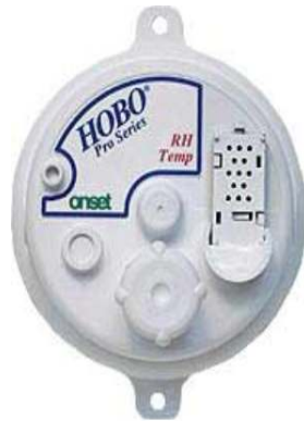
Fig. 2 Hobo sensor (Onset Corp, Southern MA, USA) for measuring temperature and humidity
