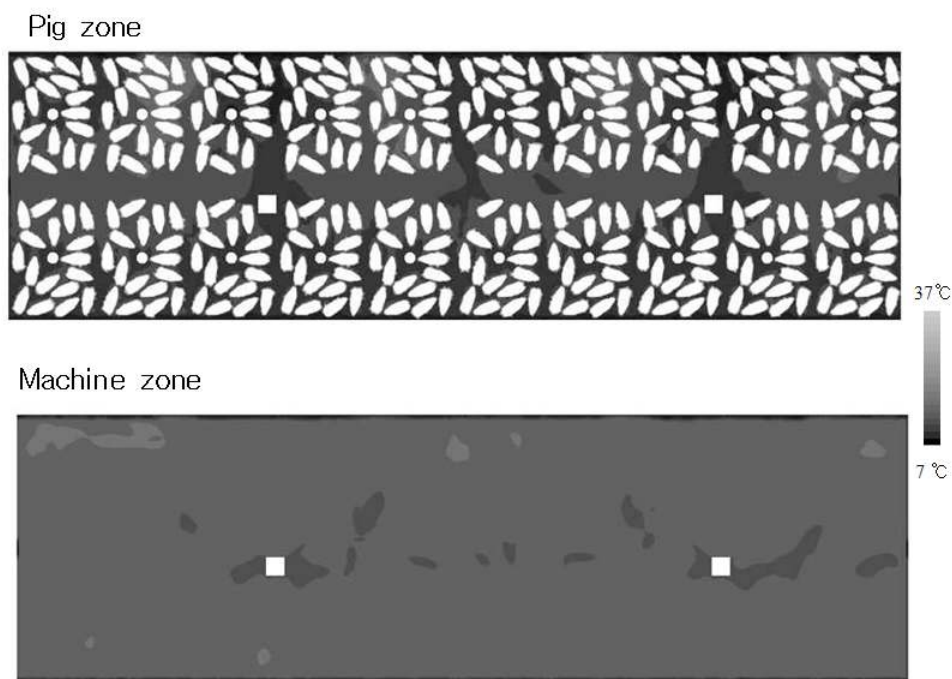
Fig. 130 Temperature distribution according to the height in case 5, pig house C
