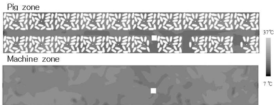
Fig. 90 Temperature distribution according to the height in case 3
