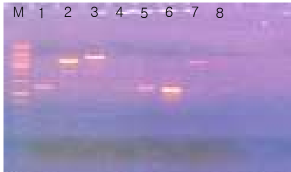
Fig. 34. Restriction analysis of gD clone 4 and expression vector. M: DNA size marker; lane 1: cutted insert gD; lane 2: cutted Pqe30; lane 3: cutted pqe-gfp; lane 4,5,6: PCR product; lane 7,8: vector.
