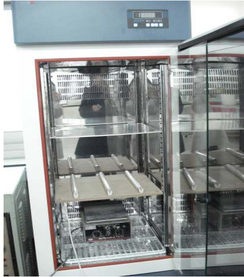
Figure 3-1. Light box for singlet oxygen generation
