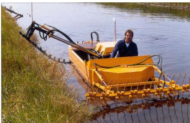
(그림2-10) Rake type Small mowing boat type
