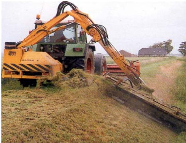
(그림2-7) Frail mower type
