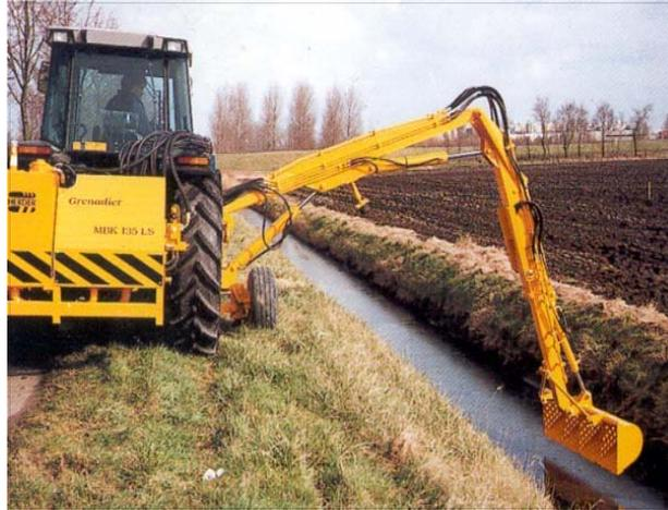
(그림2-6) Mowing Bucket Type
