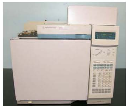
Figure 8-11. MIDI SHERLOCK system software and 6890N gas chromatograph (Agilent, USA)
