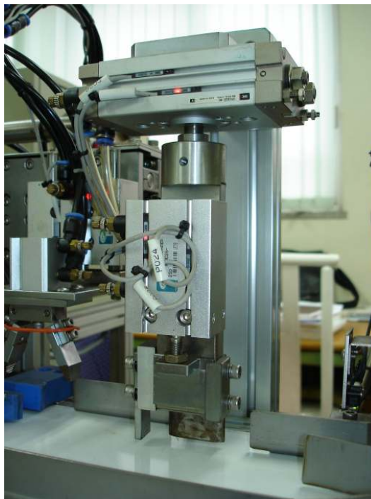
Fig 15. A turning tunit of chicken foots (90°)
