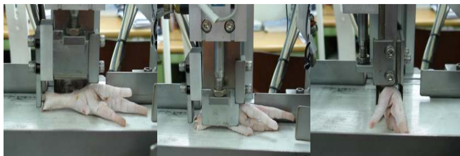
Fig 16. A picture of turning chicken feet by turning unit.
