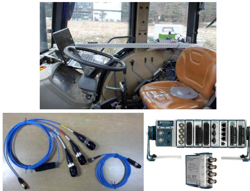
그림 3.4.17 WBV measurement instrumentation at operator's seat (left), and accelerometers and data acquisition system (right)
