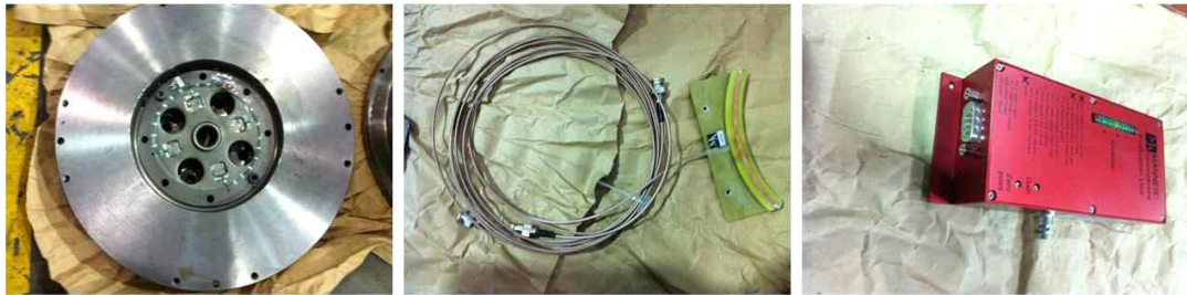
(a) Strain gage+rotor antenna (b) Stator antenna (c) Reciever
