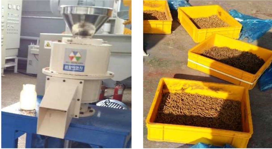
Fig. 3-12. 펠릿성형기와 결과물 (Pellet Press and Pellets of mushroom spent media)
