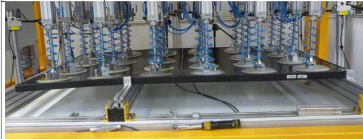
Figure 9: Photo of a module tested using CL1a_650/20 mounting option.
