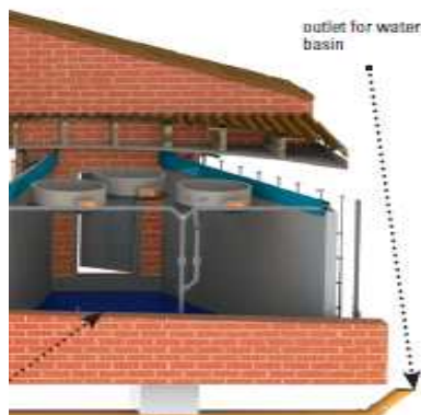
High-quality plastic pads are sprayed with water → dust does not adhere
