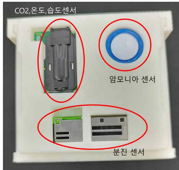
Figure 5. Bottom view of integrated sensor module without bottom cover
