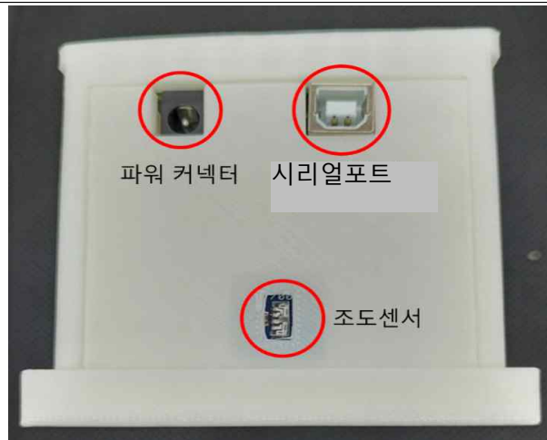
Figure 4. Top view of integrated sensor module
