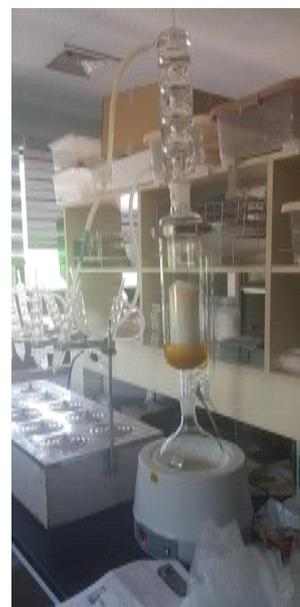
Fig. 14. Black soldier fly larvae meal manufactured by Dongeuibogam Co. (주동의보감) Fig. 15. Soxhlet extraction for elimination of oils from Black soldier fly larvae meal.
