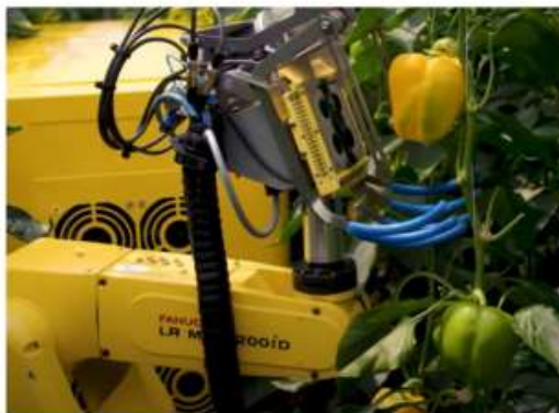
Fig. 1. A harvesting robot, SWEEPER of [1-2]. SWEEPER is used for sweet pepper harvest.
