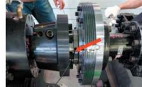
Fig. 4. A photo of the receiver to collect data from the rotating body in real time
