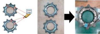
Fig. 3. A photo of sprocket with strain gage to measure driving torque
