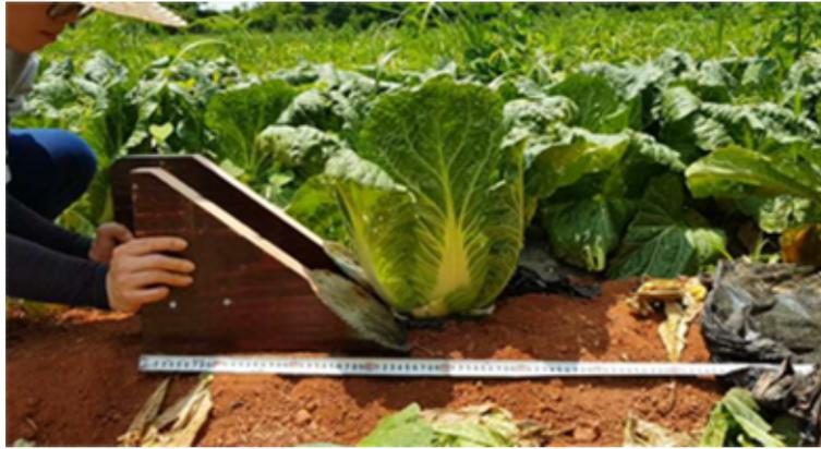
그림 48 Experiment to find the effect of a preprocessing unit on the pushing behaviour of Chinese cabbage
