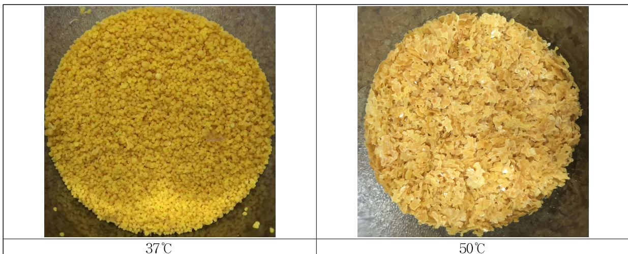
Fig 5. Change of bead shape according to drying temperature.
