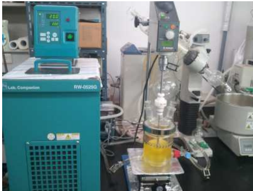
Figure 42. Bulk-scale batch mode reactor used for acidolysis reaction of PC with DHA
