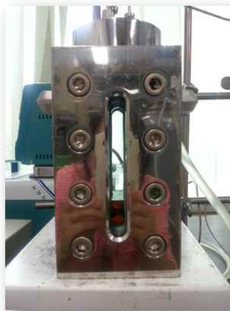
Figure 47. Water jacketed high pressure vessel
