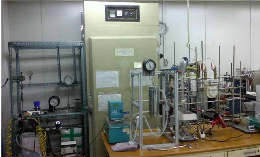
Figure 63. Supercritical carbon dioxide extraction system used in the present study.
