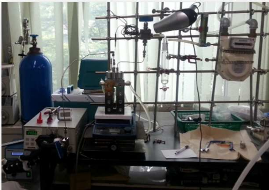
Figure 22. Supercritical carbon dioxide system for fatty acid extraction
