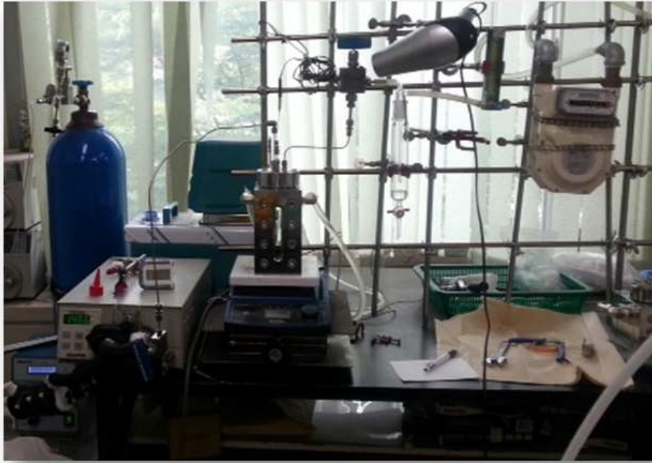
Figure 46. Supercritical carbon dioxide system for fatty acid extraction
