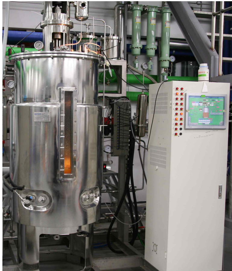
Figure. 99. Bulk scale reaction system for production of Reconstituted phospholipid by enzymatic esterification.
