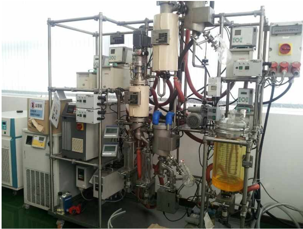
Figure. 101. Distillation Tower within Optimized Packing Material for Purification of Medium Viscosity Lecithin
