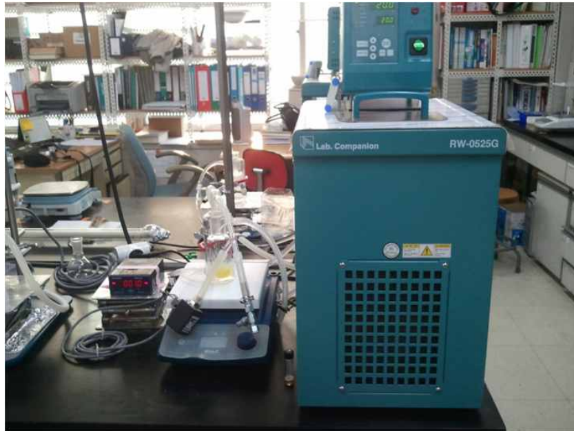
Figure 44. Water jacketed batch reactor for enzymatic reaction under vacuum.
