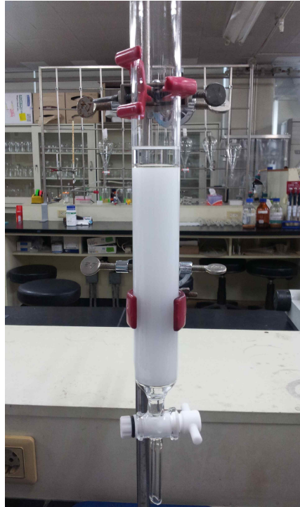
Figure 71. Silica column chromatography to remove residual FFAs and phosphocholine from reaction products
