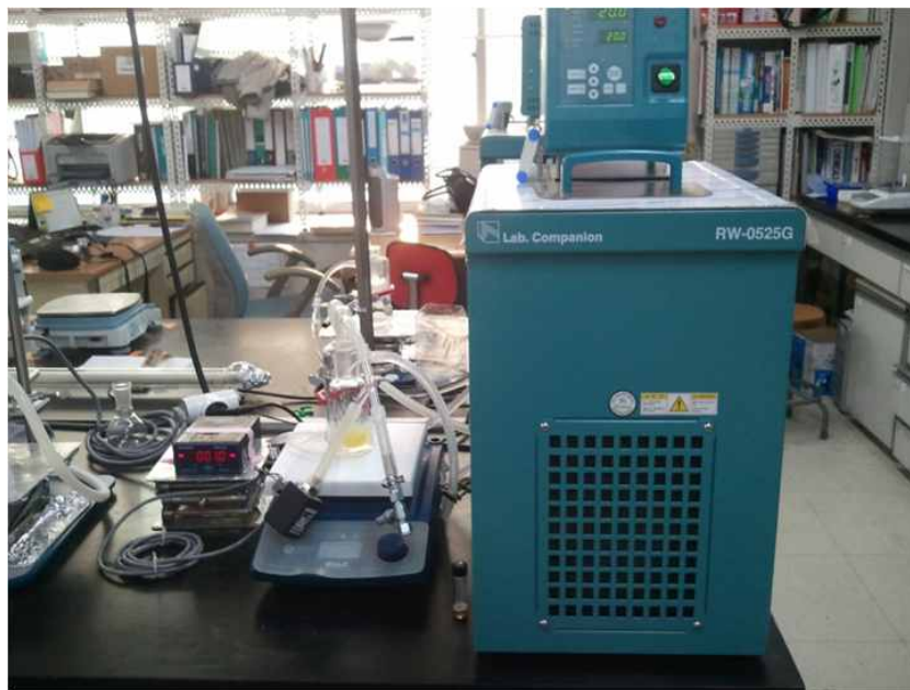
Figure 4. Water jacketed vacuum reactor for enzymatic reaction
