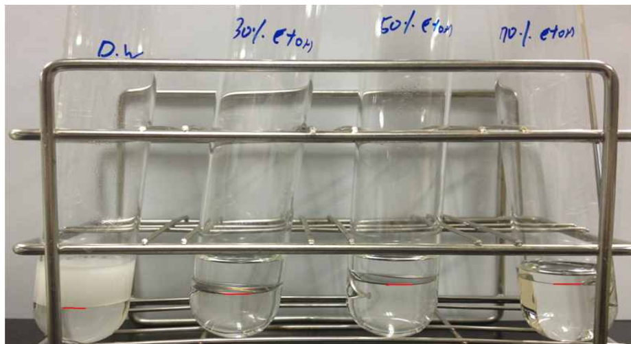
Figure 68. Aqueous ethanol/dichloromethane extraction of sn -1 lysophosphatidylcholine from reaction products. The concentrations of aqueous ethanol were 0, 30, 50, and 70%.
