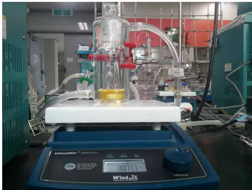
Figure 3. Water jacketed batch reactor for enzymatic reaction.
