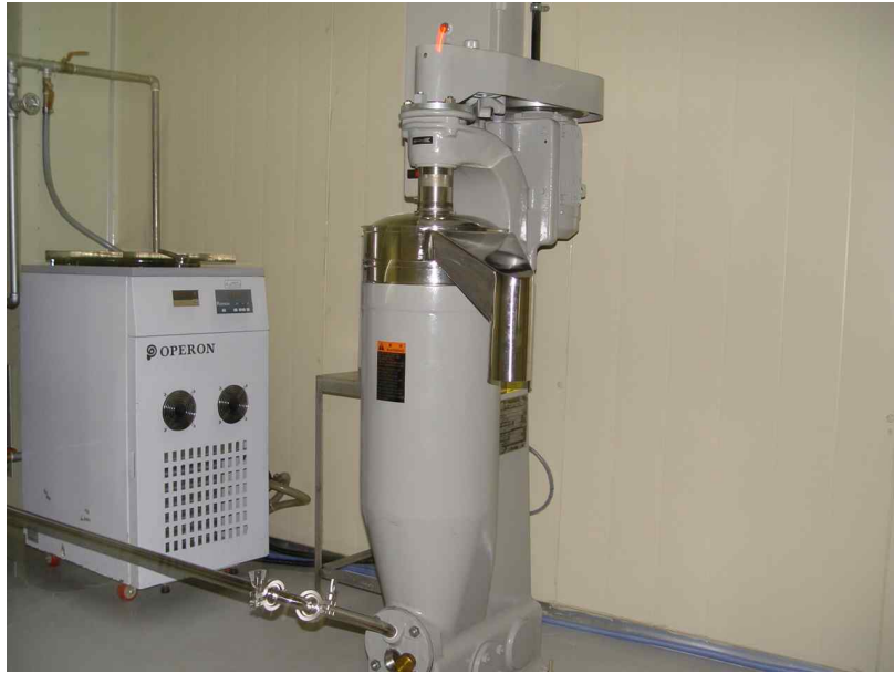
Fig. 58. High speed centrifuge for Cell Harvest
