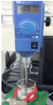
Fig. 3. Apparatus set up for the determination of solubility.
