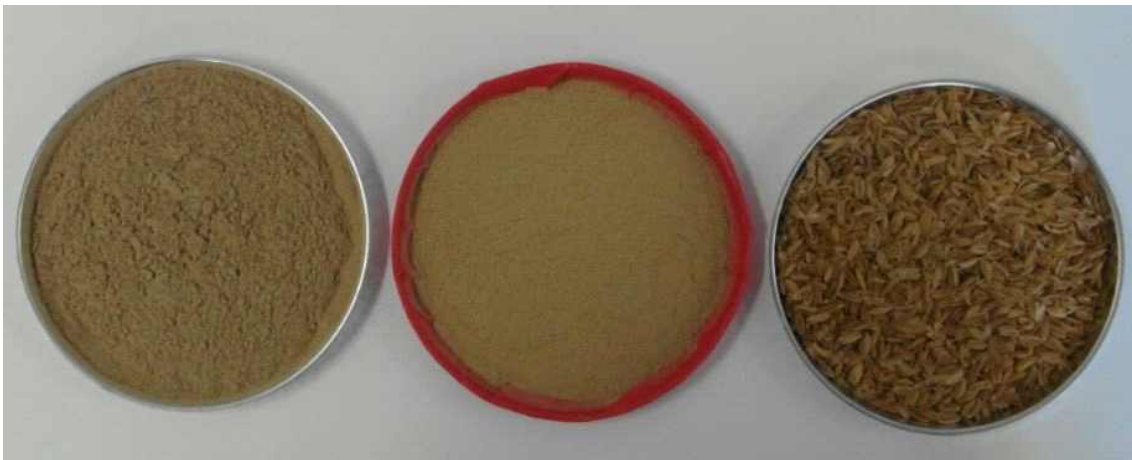
Fig. 3.207. Appearance and color of commercial wood powder(left), rice husk organic filler (middle), rice husk(right) after 8 days of humid heating aging.
