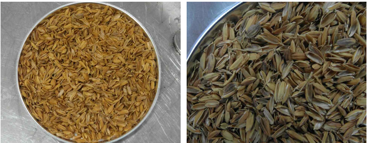
Fig. 3.214. Magnified images of rice husk after 20 days of humid heating aging.
