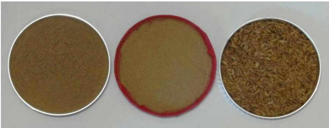
Fig. 3.210. Appearance and color of commercial wood powder(left), rice husk organic filler (middle), rice husk(right) after 14 days of humid heating aging.
