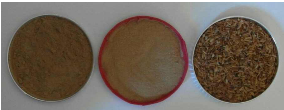
Fig. 3.211. Appearance and color of commercial wood powder(left), rice husk organic filler (middle), rice husk(right) after 16 days of humid heating aging.
