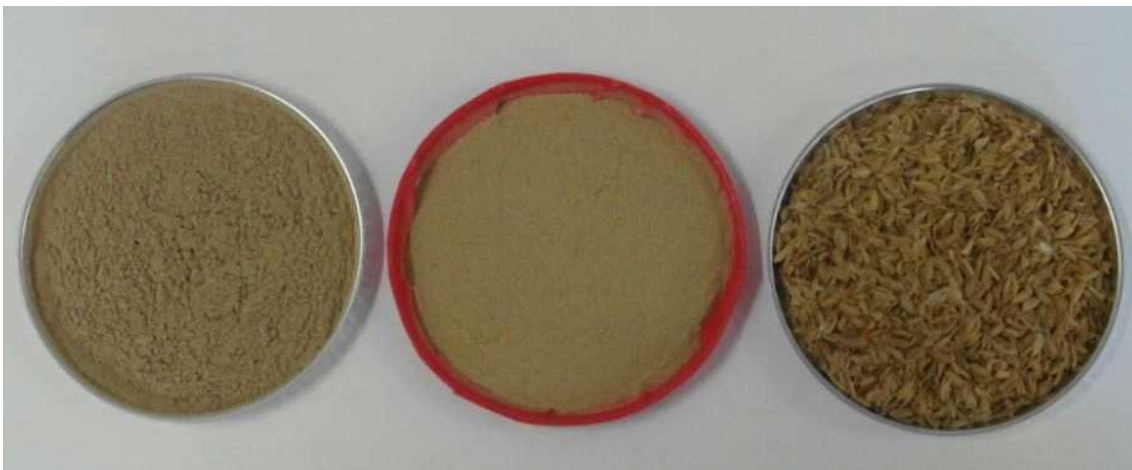
Fig. 3.204. Appearance and color of commercial wood powder(left), rice husk organic filler (middle), rice husk(right) after 2 days of humid heating aging.
