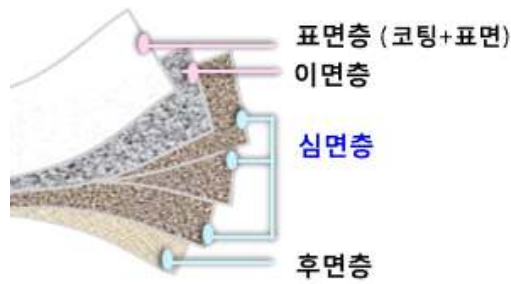
Fig. 3.198. Structure of duplexboard.
