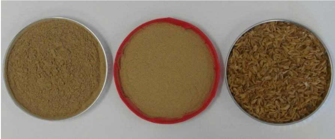
Fig. 3.206. Appearance and color of commercial wood powder(left), rice husk organic filler (middle), rice husk(right) after 6 days of humid heating aging.
