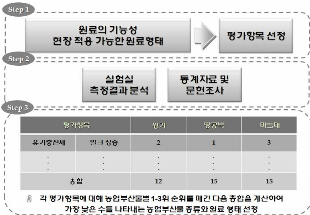
Fig. 3.175. Flow diagram of the evaluation of agricultural byproducts.
