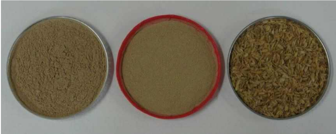
Fig. 3.203. Appearance and color of commercial wood powder(left), rice husk organic filler (middle), rice husk(right) before humid heating aging.
