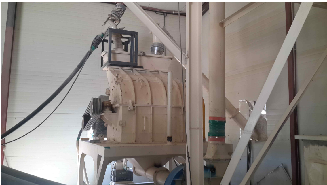
Fig. 3.177. Grinder for the production of organic filler.
