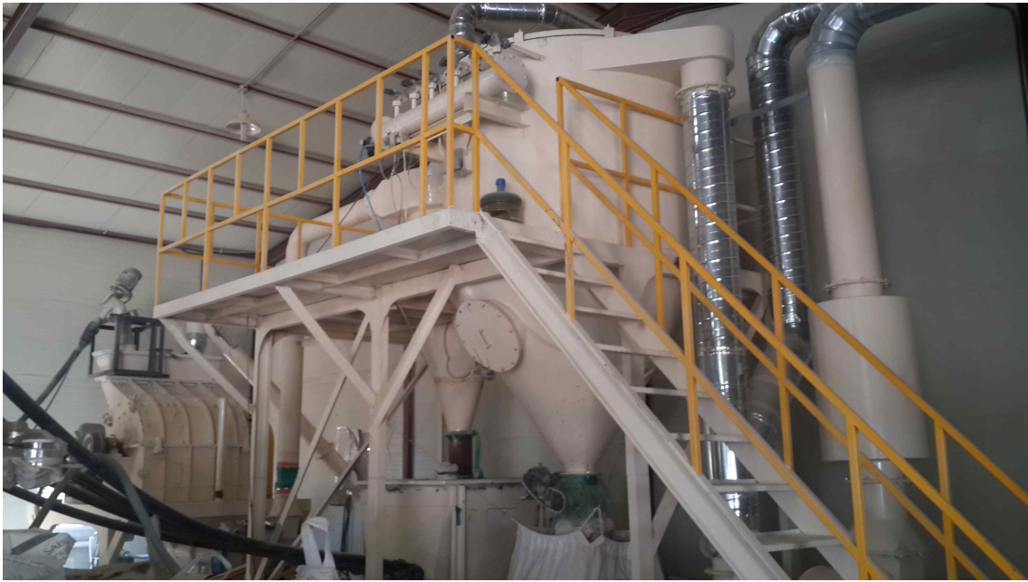
Fig. 3.176. Dryer for the production of organic filler.
