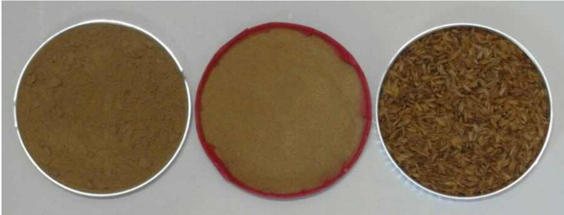
Fig. 3.212. Appearance and color of commercial wood powder(left), rice husk organic filler(middle), rice husk(right) after 18 days of humid heating aging.
