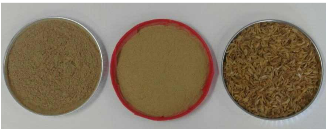
Fig. 3.205. Appearance and color of commercial wood powder(left), rice husk organic filler (middle), rice husk(right) after 4 days of humid heating aging.
