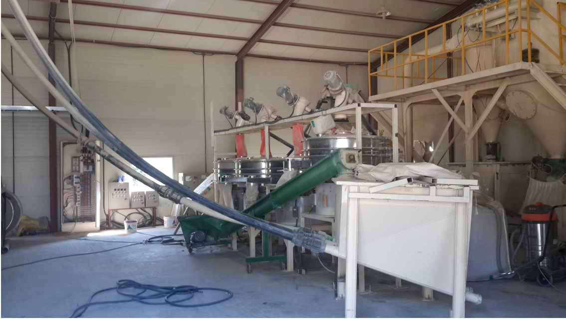
Fig. 3.178. Screens for the production of organic filler.
