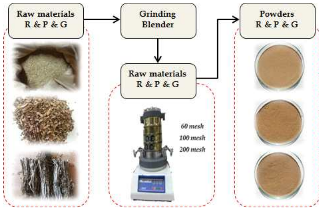
Fig. 3.8. Manufacture of the agricultural byproducts organic fillers.
