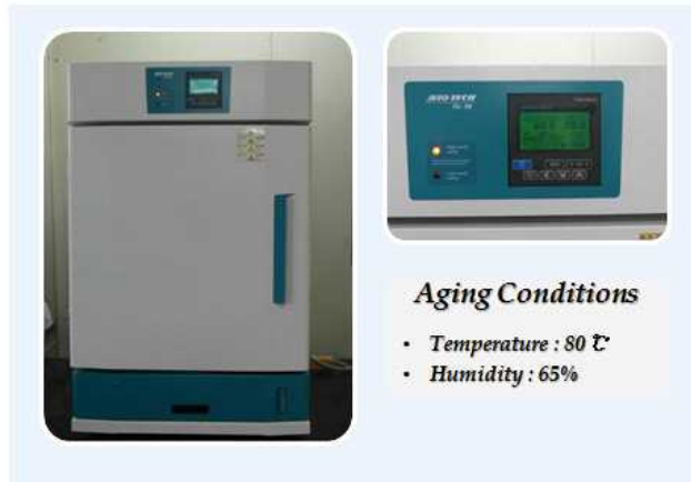
Fig. 3.202. Thermo-hygrostat and aging conditions.
