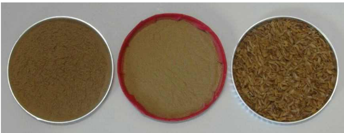
Fig. 3.208. Appearance and color of commercial wood powder(left), rice husk organic filler (middle), rice husk(right) after 10 days of humid heating aging.
