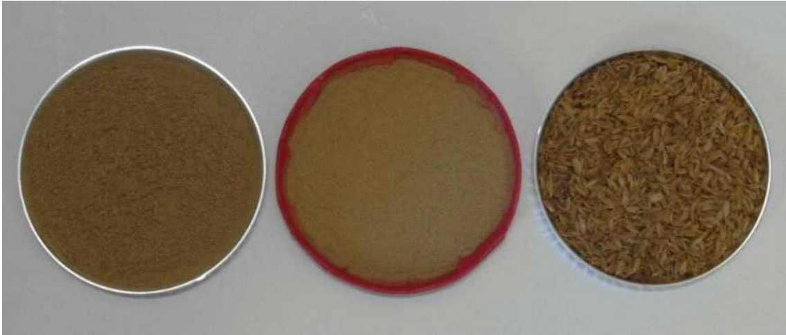
Fig. 3.209. Appearance and color of commercial wood powder(left), rice husk organic filler (middle), rice husk(right) after 12 days of humid heating aging.
