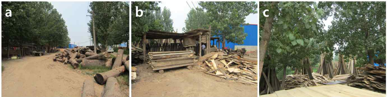
Figure 3-30. Log of Paulownia (a), sawing of log (b) and air drying of boards (c) in CN-C
