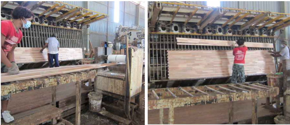
Figure 3-15. Manufacturing process of laminated board in MY-B
