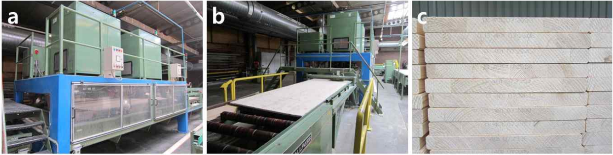
Figure 3-40. High frequency gluing process of laminated board in NL-A (a and b) and labeling of manufacturing information of laminated board (c)
