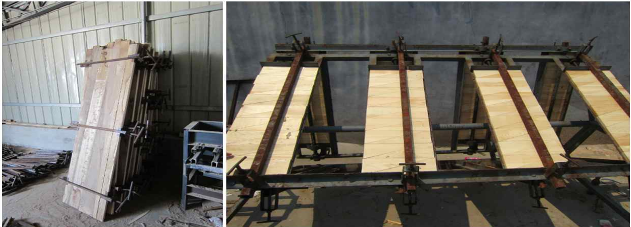
Figure 3-34. Manufacturing process of laminated board in CN-B
