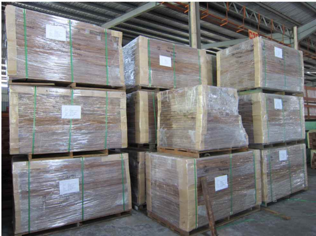
Figure 3-20. Example of packaging of laminated board for export to European countries in MY-A
