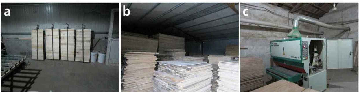
Figure 3-36. Manufacturing process of laminated board in subcontractor of CN-D (a), storage of laminated board from the subcontractor in CN-D (b), and planing of laminated board in CN-D (c)
