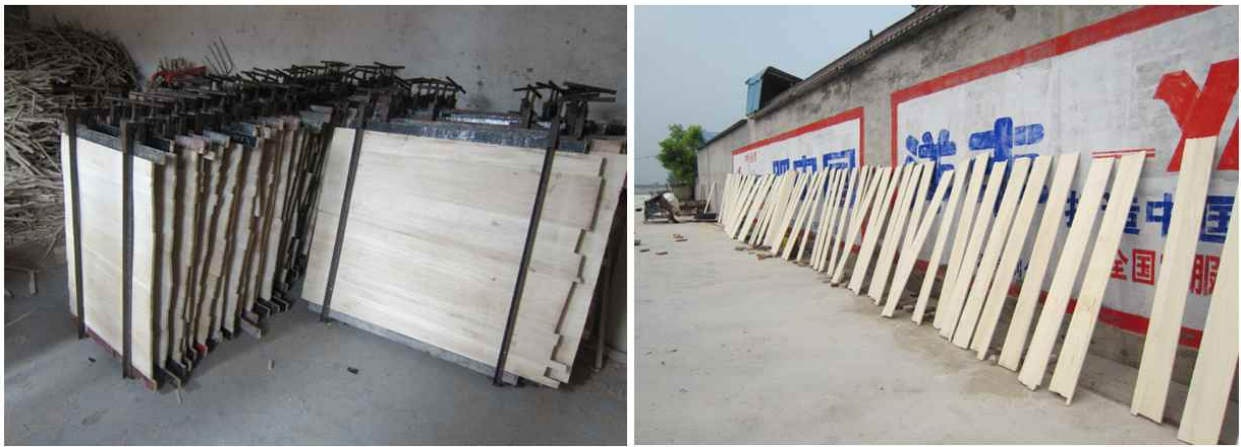
Figure 3-35. Manufacturing process of laminated board in CN-C (left) and bleaching of laminated board with hydrogen peroxide
