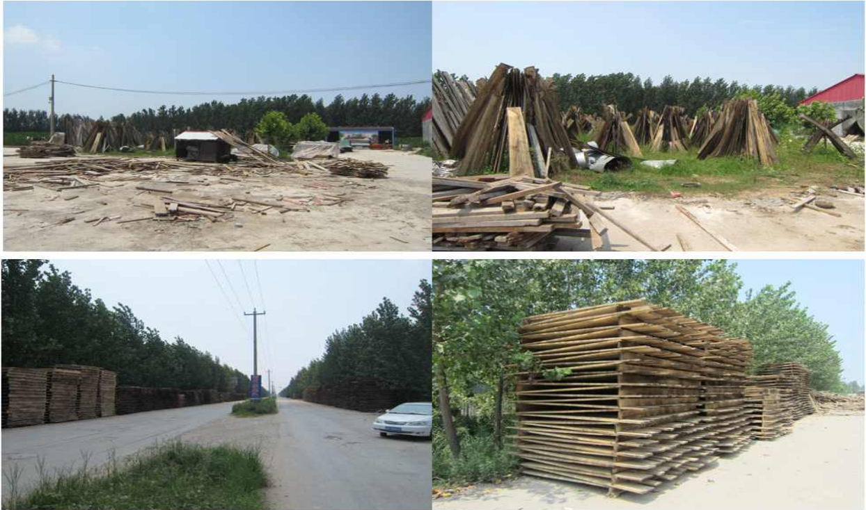
Figure 3-29. Air drying of Paulownia in CN-B
