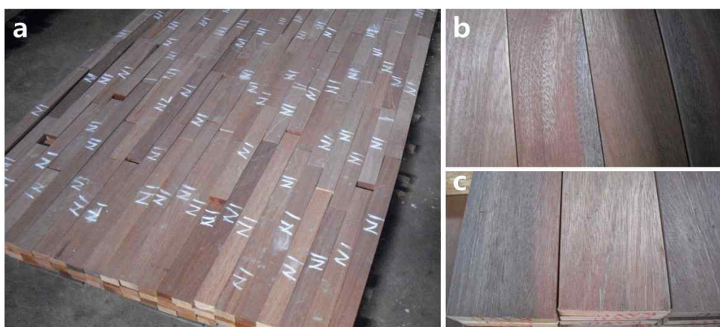
Figure 3-14. Laminae prepared for manufacturing of laminated board (a, for export to European countries; b, for export to Korea)
