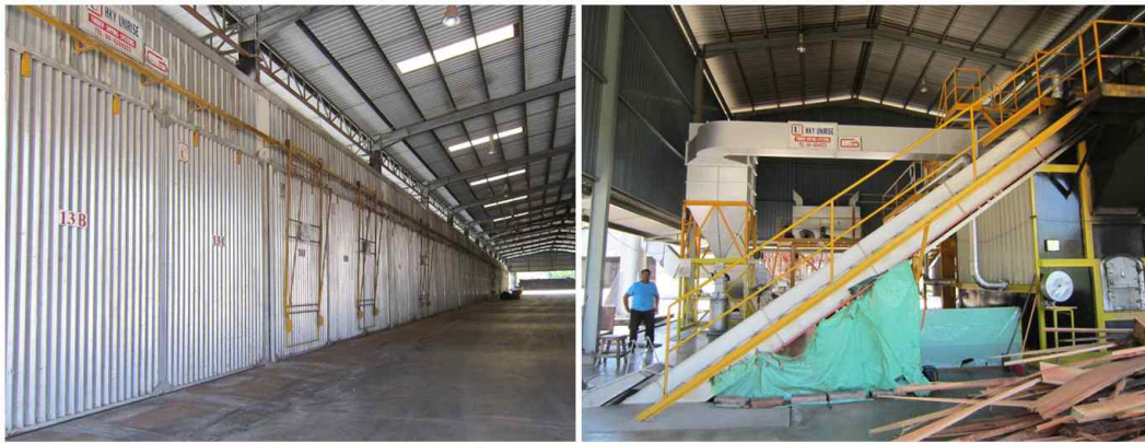
Figure 3-8. Kiln drying system for laminae in MY-A
