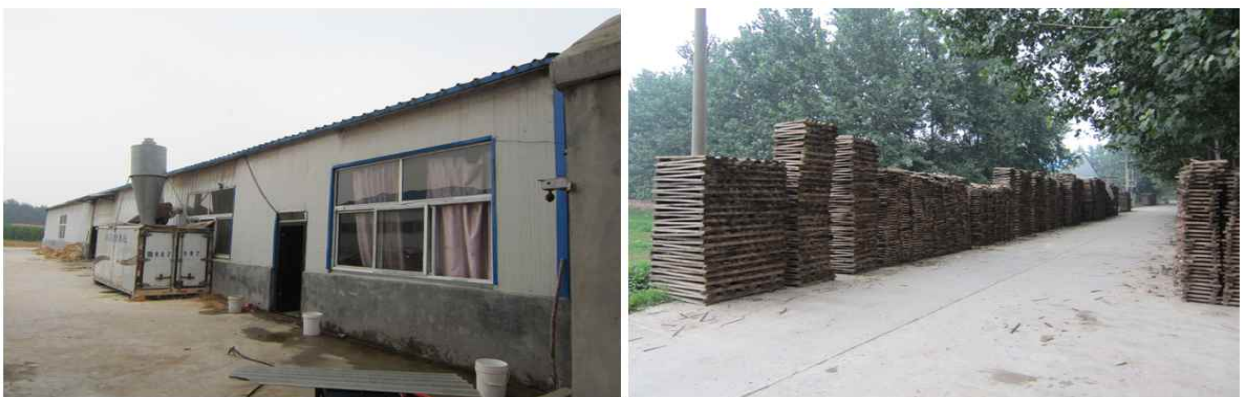
Figure 3-31. Subcontractor of CN-D (left) and air drying of Paulownia in the Subcontractor (right)
