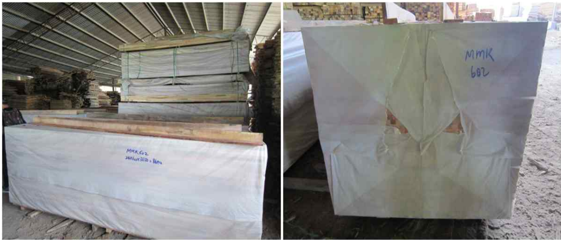
Figure 3-22. Packaging of laminated board in MY-C
