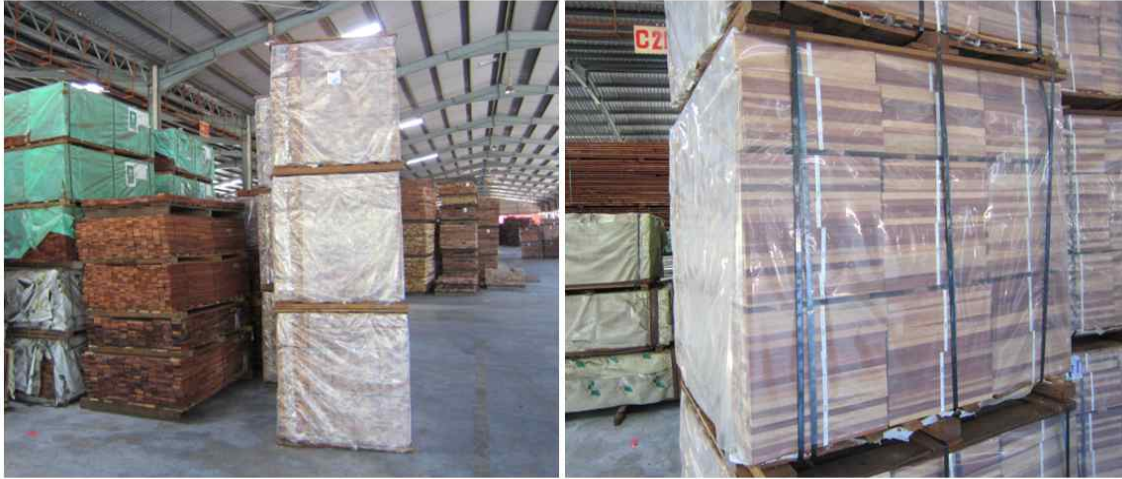
Figure 3-17. Packaging of laminated board in MY-A
