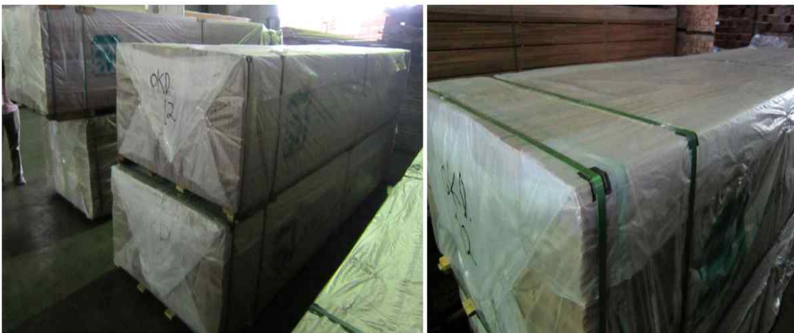
Figure 3-23. Packaging of laminated board in MY-D
