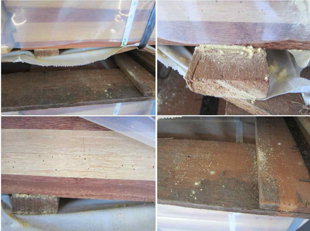
Figure 3-19. Exit hole and frass by insect on surface of packed laminated board in MY-A
