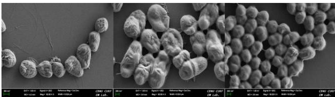
Fig. 42. Field emission scanning electron micrograph of SCWL 08(right), SCWL 10(middle), SCWL 20(left).
