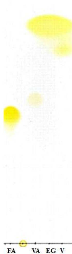
Fig. 49. TLC chromatogram of standard compounds, ferulic acid(FA), 4-ethylguaiacol(4-EG), vanillin(V) and vanillic acid(VA), for the screening of flavor producing yeast strains.
