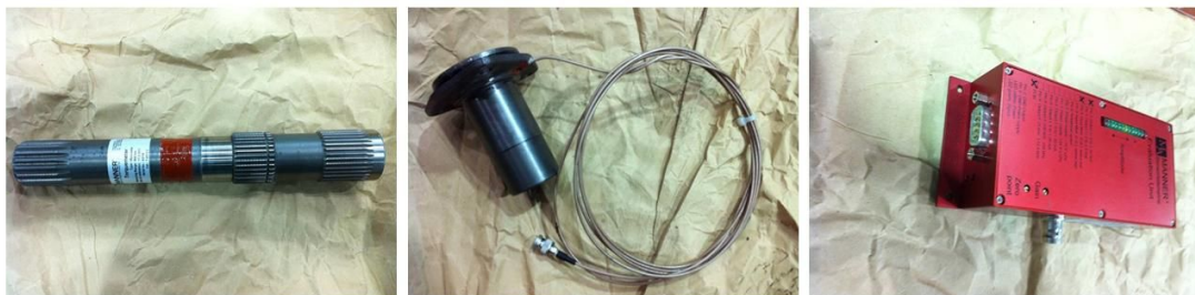
(a) Strain gage+rotor antenna (b) Stator antenna (c) Receiver
