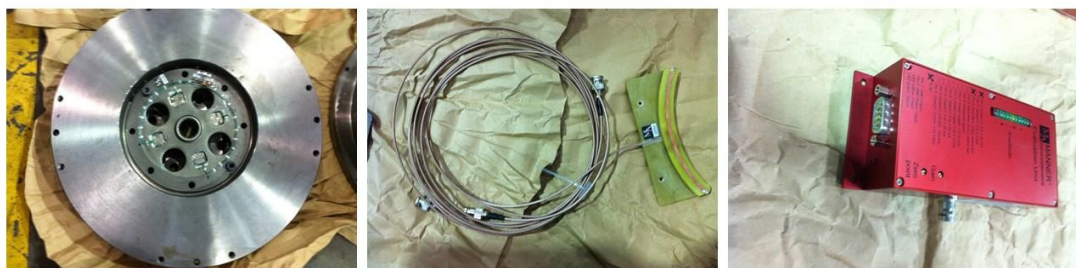
(a) Strain gauge+rotor antenna (b) Stator antenna (c) Receiver
