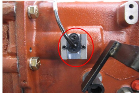
(b) Proximity sensor for measuring transmission revolution speed
