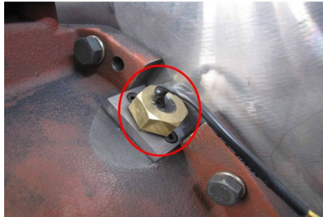
(a) Proximity sensor for measuring engine revolution speed
