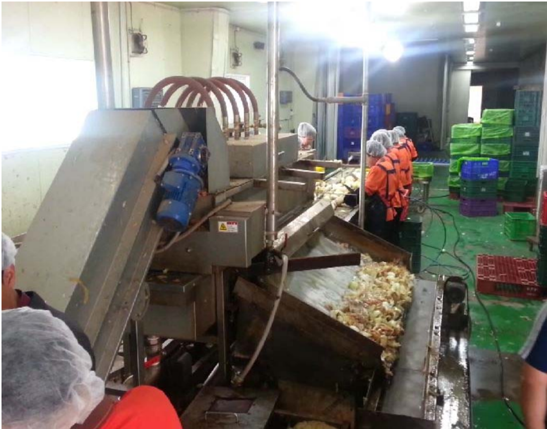
그림 19. Water injection type onion peeling machine : large area, a lot of energy
