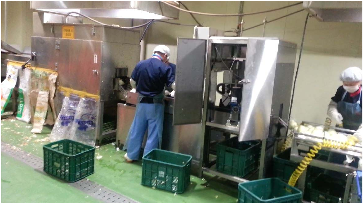
그림 18. Compressed air injection type onion peeling machine : large area, a lot of energy
