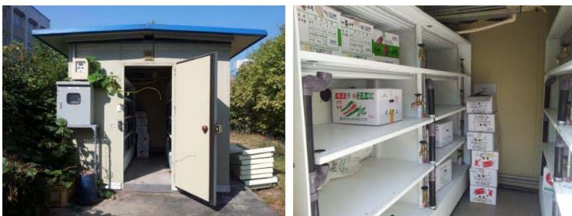
Fig. 50 Low temperature storage system of red pepper used in the experiment.
