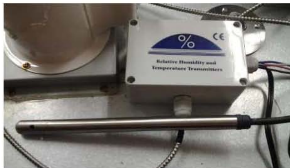
Fig. 20 Photo of the temperature and relative humidity sensor used for the test
