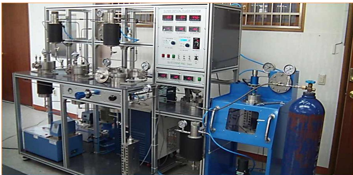
Fig. 8 Schematic diagram of the pilot-scale supercritical fluid extractor used in this study.
