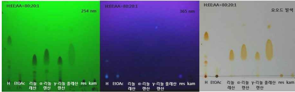
Fig. 35. Thin layer chromatography (TLC) of hexane fraction and ethyl acetate fraction from Tenebrio molitor
