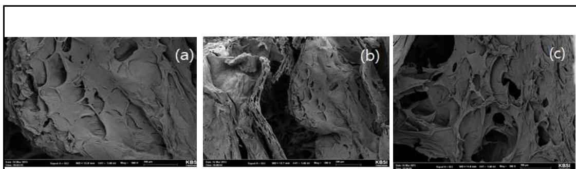
Fig. 21. Scanning electron microphotographs of the surface of Citrus after treating high pressure process for 5 minutes, 15 minutes and only water extract.
