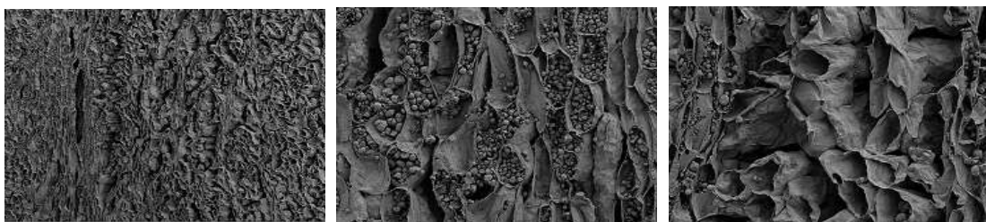
Fig. 25. Scanning electron microphotographs of the surface of sweet potato after treating high pressure process for 5 minutes, 15 minutes and only water extract.
