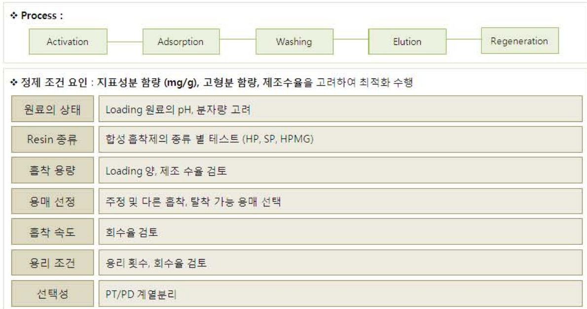
Figure 5. Process flow and considered factors of purification
