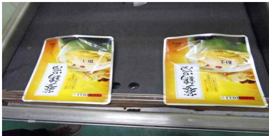
Fig. 13. Vacuum packaging of retort pack Chuncheon Dakgalbi.
