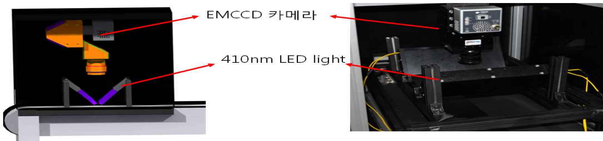
그림 9. LED lighting sources and image acquisition parts of the online multi-spectral imaging system
