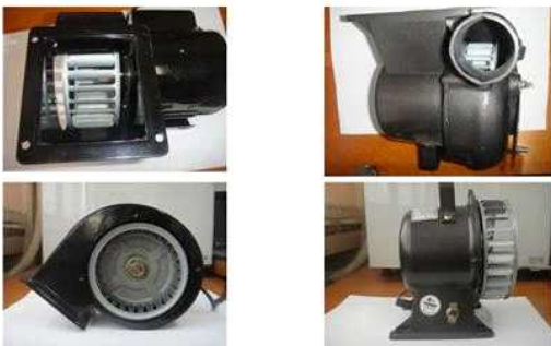
그림. 2 Types of forward centrifugal fans for experiment
