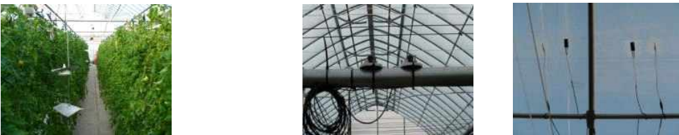
그림. 3. Air temperature, humidity, PPF and heat flow sensors installed in experimental greenhouse
