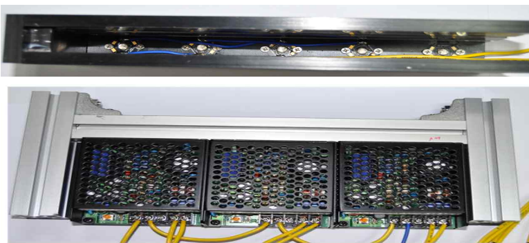
그림 8. Photos of the inside of lighting source and its power supply unit
