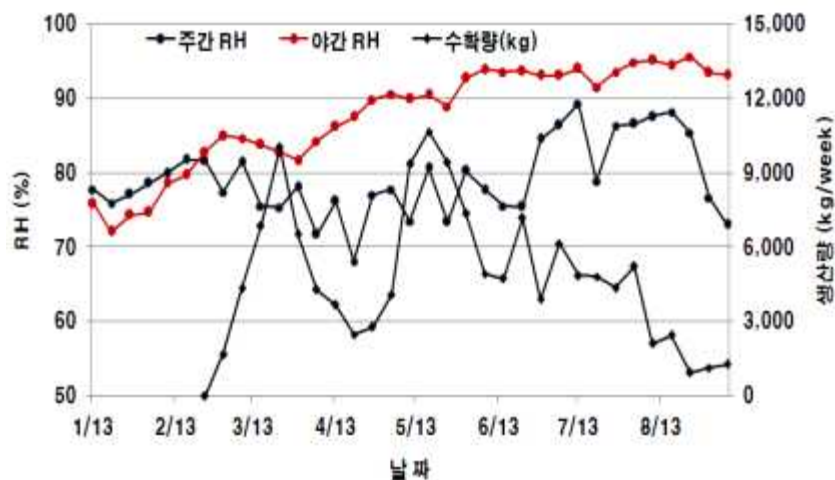
[그림 3-I-14]. Humidity and yield of paprika's green house without air duct facility
