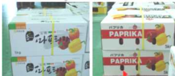
There are panel vent to pre-cool products.
