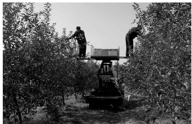
그림 2-138. Scene of working on the balance-controlled platform lifting utility.
