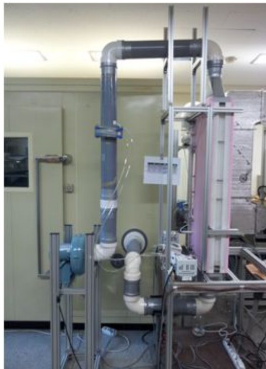
Fig. 3.5.7 OA to SA flow path connection
