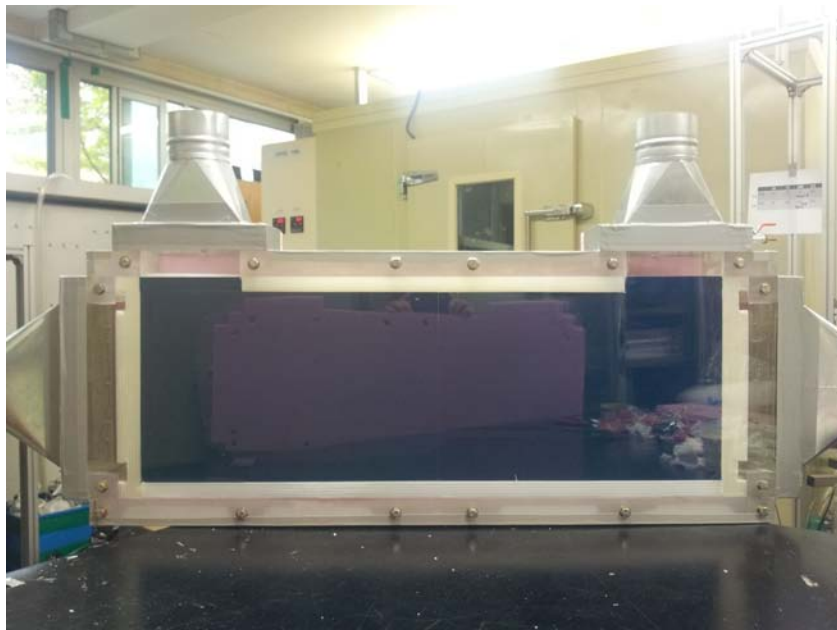
Fig. 3.5.10 Acrylic frame for fixing the heat exchanger element
