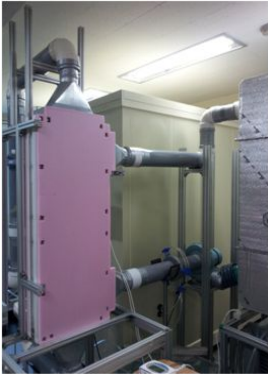
Fig. 3.5.8 RA to EA flow path connection
