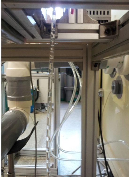
Fig. 3.5.9 Drainway of heat exchanger element
