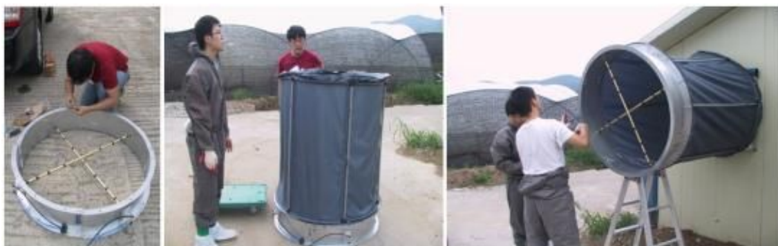
Fig. 3.1.4. Measuring flow rate of ventilation fan of broiler house
