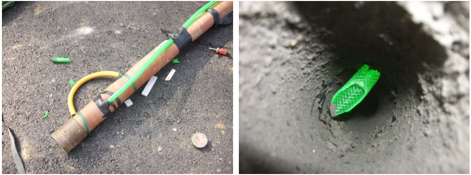
Figure 52. The modification of air gun hose to increase the stickiness of soil material (green hose was for water supply).
