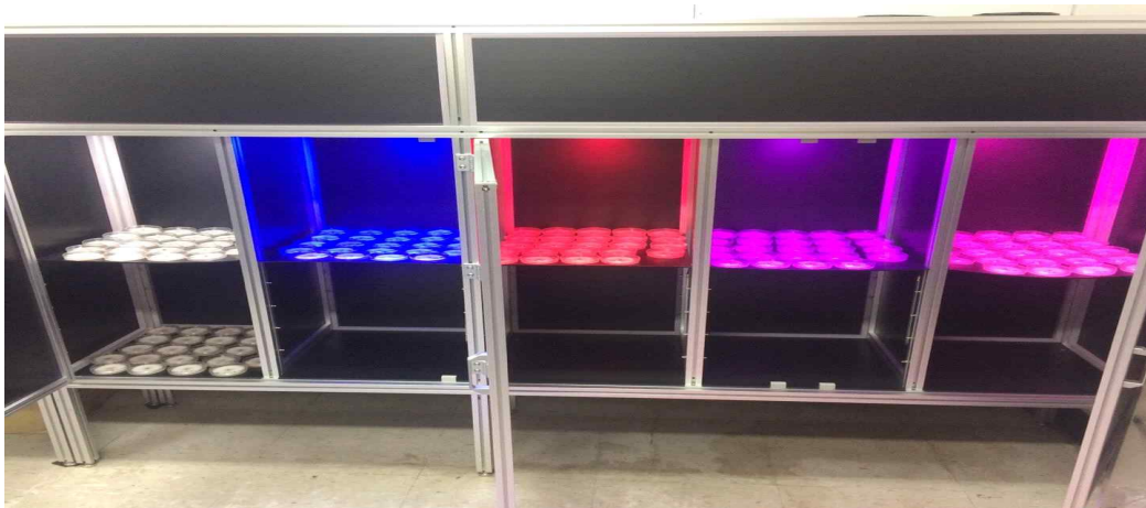
[그림 237] Chamber with different light conditions including QD-LED.
