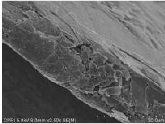
(b) Expandable Graphite(S2 grade, Size: 420um, Expansion Ratio: 250%)
