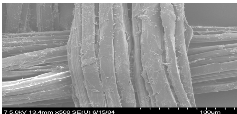
Fig. 27. SEM photograph of mordanted silk fabric by iron sulfate.
