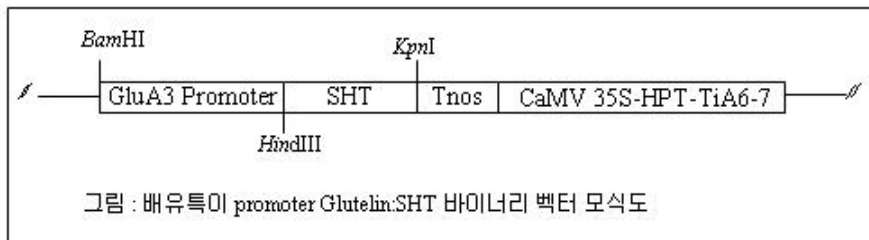
Fig. 2-1. Schematic diagram of binary vector pGA1611 harboring SHT gene under the control of rice glutelin A3 promoter
