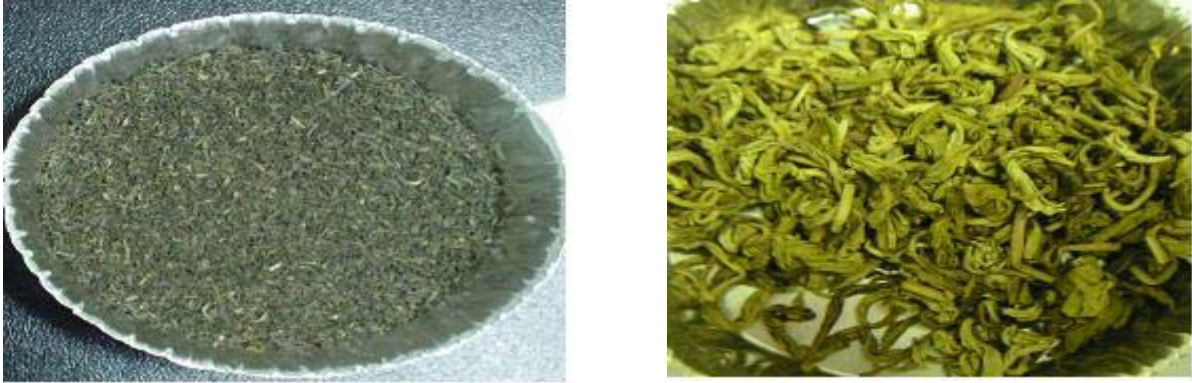
Fig. 2.6. Comparison of untreated (left) with treated(right) by SC-CO 2 at flow rates 5.5 g/min, 300 bar, and 70 °C for 480 min. Particle size of green tea was 5,500 ~ 17,400 μm (no grinding). Extraction cosolvent was 5.8% of g EtOH per g CO 2 .
