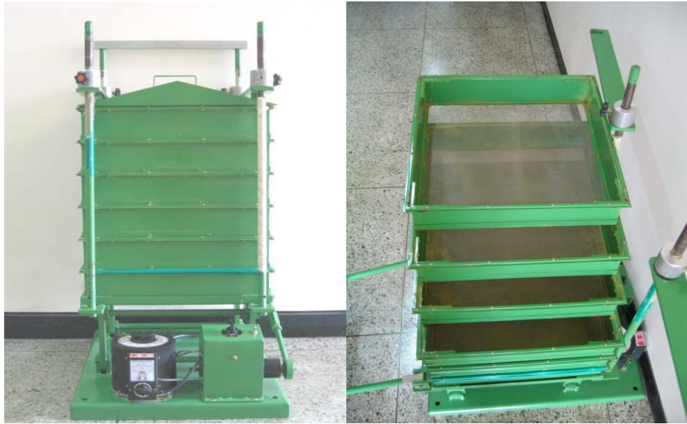
Fig. 21. Machine for pollen refining.
