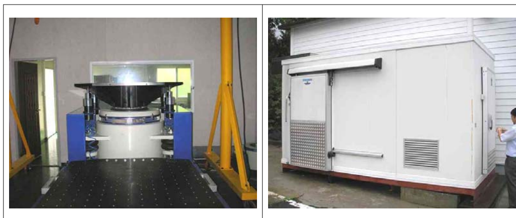
Figure 87. Vibration Tester and Environmental Chamber.
