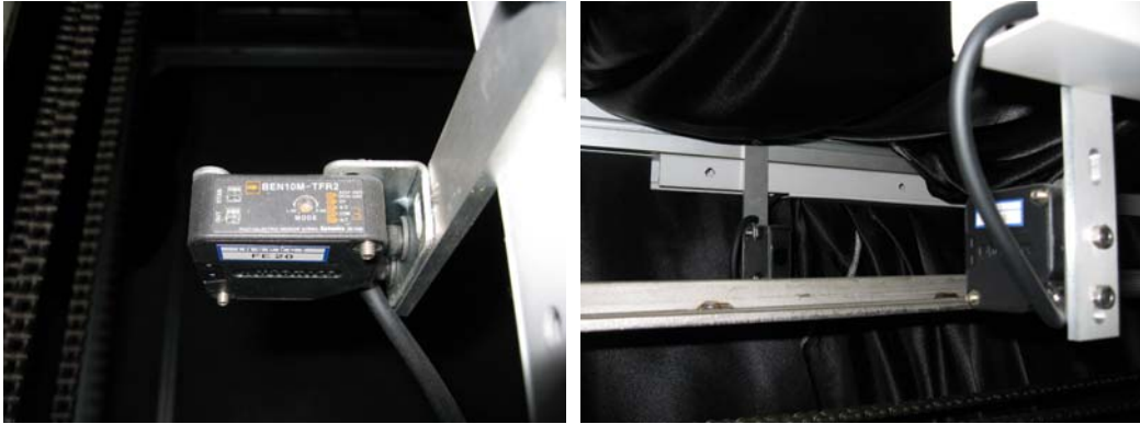
Fig 3-2-6. Photo sensor of change motor direction
