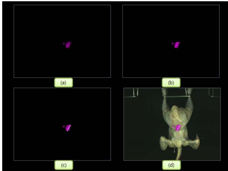
Fig. 3-4-48 (a) Bruise blobs isolated out of background, (b) After dilation and erosion operator, (c) The longest diameter in breast part, (d) Superimposing onto the raw image.
