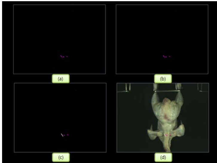
Fig. 3-4-52 (a) Bunches of extra-feather isolated out of background; (b) After dilation and erosion operator, (c) The longest diameter in breast part, (d) Superimposing onto the raw image.
