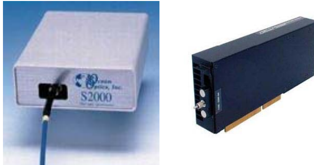
Fig. 8 Outlook of spectrophotometers (S2000 and CDI).
